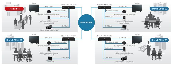
Example of standard point to point connection with the KX-VC1000 Activation Key (sold separately, see page 15) expands the function to enable 4-site connection.
