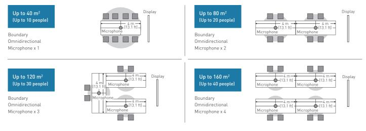
\*This diagram is intended only as a layout example. It is not meant to show the maximum number of people that can be covered. \*This is the pick-up capacity when using the Boundary Omnidirectional Microphone. The capacity varies when using another microphone
